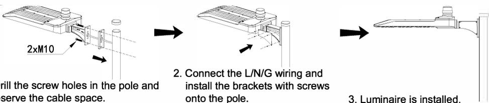
1. Drill the screw holes in the pole and reserve the cable space.
