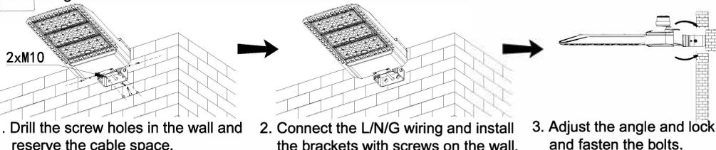
1. Drill the screw holes in the wall and reserve the cable space.
