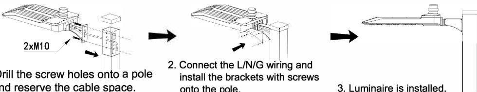
1. Drill the screw holes onto a pole and reserve the cable space.
